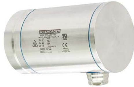
**Figure 3:** Motor H features an annealed label with a 32  $\mu$ -inch surface finish. Unlike etching, the annealed label preserves the metal's surface finish. This smooth label was designed to avoid trapping bacteria or food.
